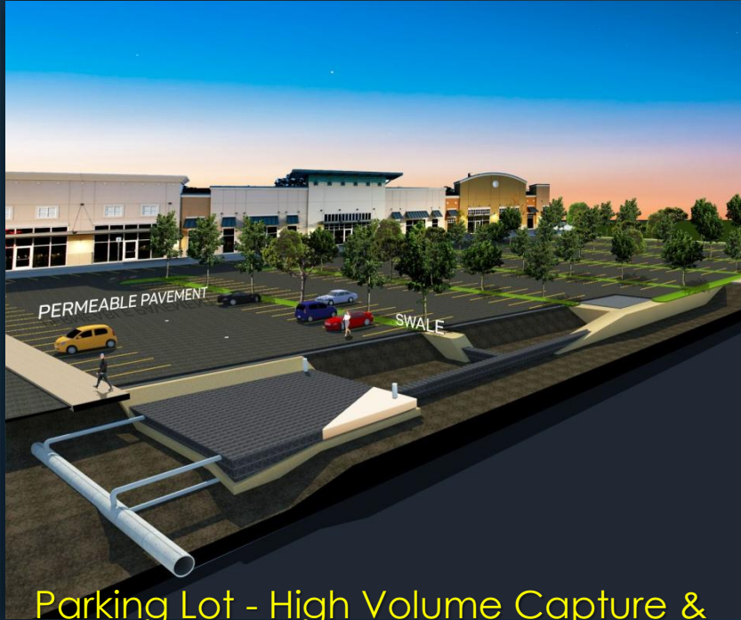
Swale with Top-Down Higher Volume Capture – and Oxygen Add to the Water
